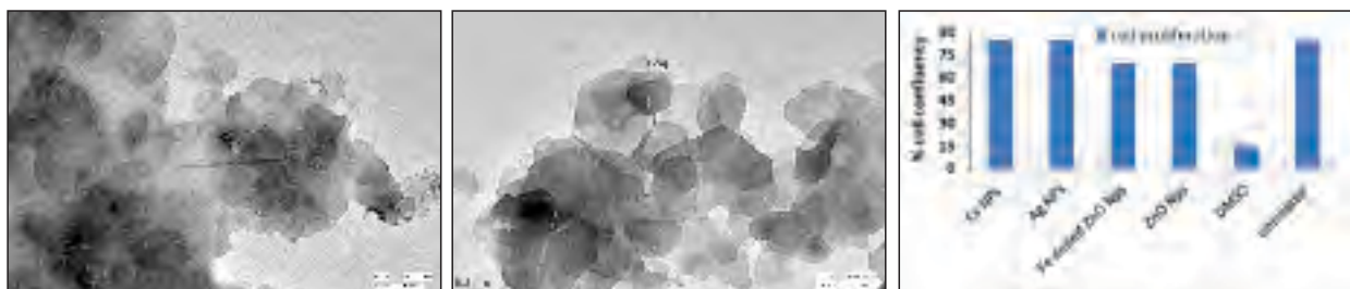
Fig.1: Morphology of ZnO Nps and Fe-doped ZnO Nps as determined by transmission electron microscopy
