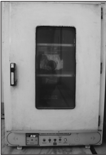
Hot air oven for hot sterilization and drying
